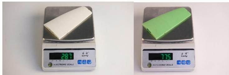
Foaming volume ratio high up to 220%, 1 roll of ePLA-LW is equivalent to 2.2 rolls of ordinary PLA.
